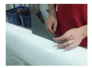
Boarder the edges of the hull and fin with masking tape, leaving 3mm (1/8") showing on the fin and the hull . Fold the ends of the tape back onto itself to ensure easy removal.
