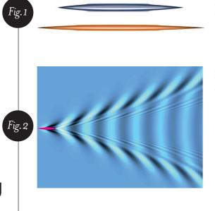
The top blue shell has a bias towards reduced frictional drag while the longer orange shell keeps wave-making drag to a minimum.
