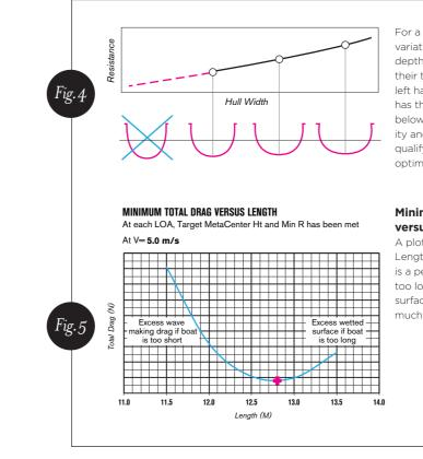
able value for the crew. So the minimum resistance is governed by the stability of the boat. In performing a length study, therefore, for each length the minimum resistance will be achieved by the narrowest boat that will still offer the required stability for the crew.
