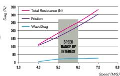
overall resistance due to wave-making drag is very small, in the order of 12% of the total at a normal racing speed of 5.5 metres/second. The initial reaction of the designer to optimising this boat might be to concentrate on keeping the wetted surface to a minimum as it is creating most of the drag. That is true but the subtlety of the trade-off of those two factors with length is very important and sometimes surprising.
